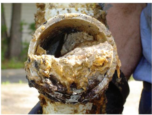
FOG is a by-product that food service establishments and residents must constantly manage. In general, FOG enters a facility's plumbing system from dish washing, floor cleaning and equipment sanitation. Sanitary sewer systems are not designed nor equipped to handle the FOGthat accumulates on the interior of the municipal sewer collection
